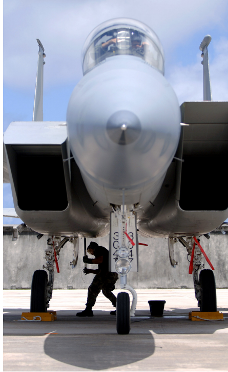
Figure 4.4: The inlet ramps of a McDonnell-Douglas F-15E Strike Eagle. Reprinted from Wikipedia.
